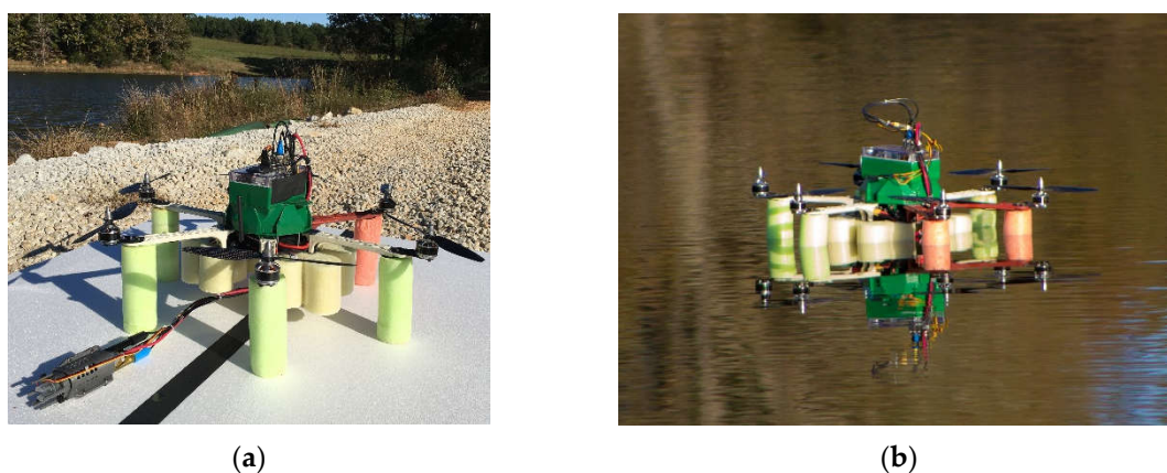
Figure 1. The unmanned aerial vehicle-assisted measurement system (UAMS): (a) prior to a flight mission; (b) floating on a water surface while making measurements.
