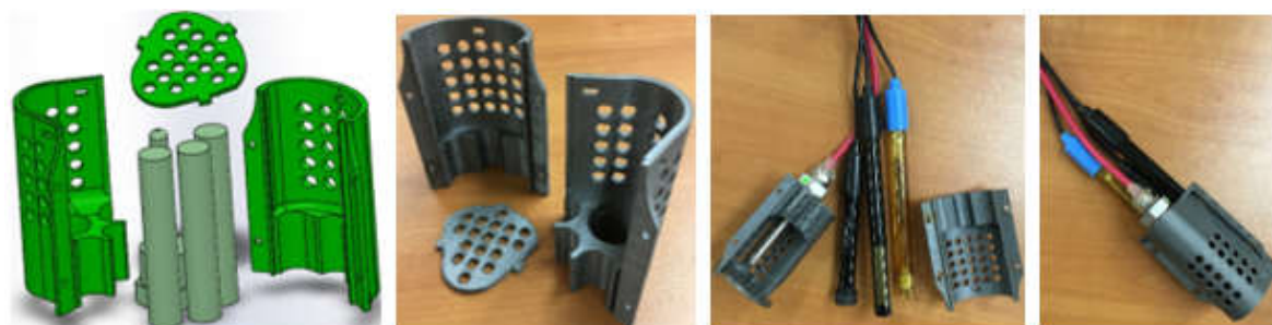
Figure 2. Custom-designed probe housing was 3D-printed with polylactic acid (PLA) material.
