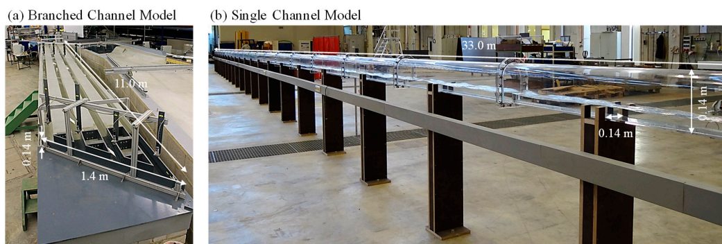
Figure 3. Photographs of the branched channel model (a) and the single channel model (b) at the Laboratory of the Institute of Hydraulic Engineering and Water Resources Management at RWTH Aachen University.
