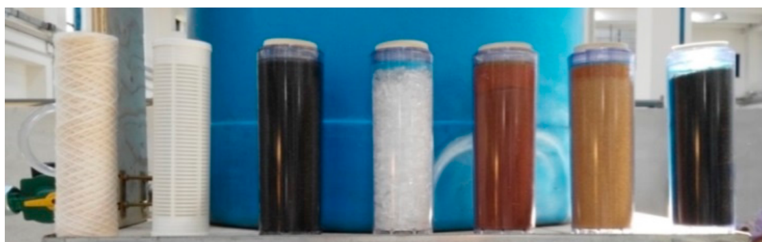
Figure 1. Filter cartridges for domestic use water that are analyzed in the present work. From left to right: 1. wire-wound polyester filter, 2. nylon mesh filter, 3. granular activated carbon filters, 4. filter cartridge with crystal polyphosphate, 5. cationic resin filter cartridge, 6. anionic resin filter cartridge, and 7. mixed-bed resin filter cartridge.
