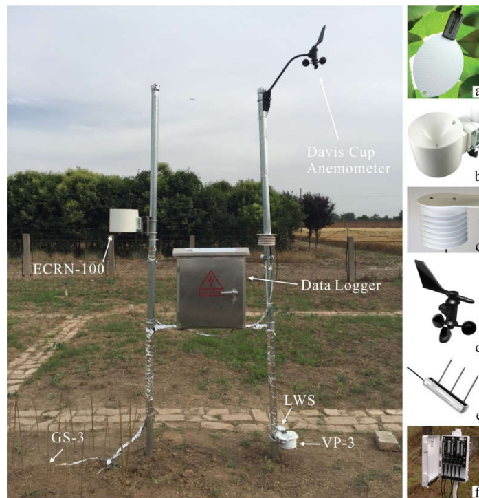
Figure 3. Filed experimental setup. Sensors include: (a) LWS; (b) ECRN-100 rain gauge; (c) VP-3; (d) Davis Cup Anemometer; (e) GS-3; (f) EM50 datalogger inside the security box.
