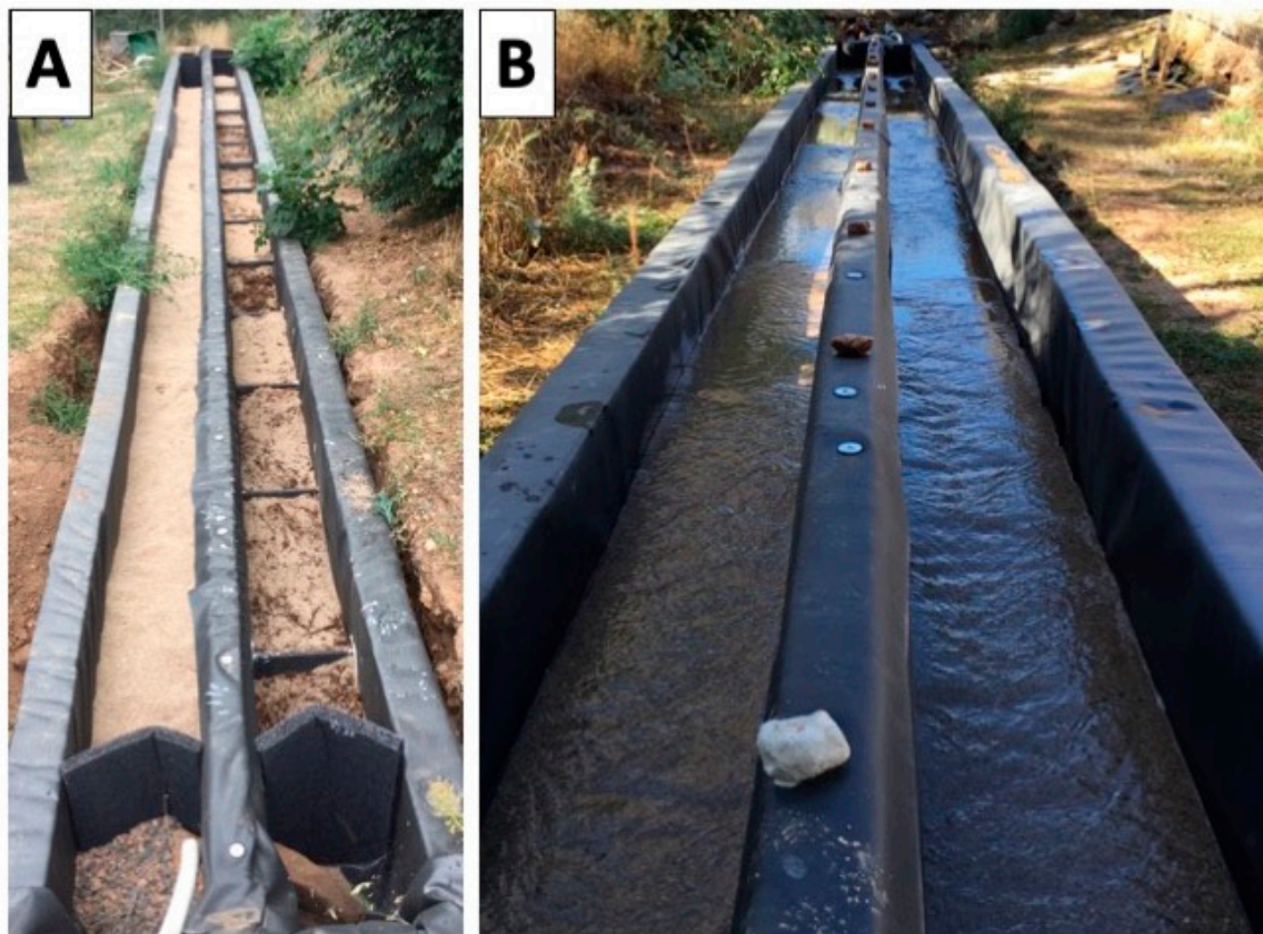
Figure 2. Photos from constructed streams showing (A) triangular BEST modules and sand/woodchip geomedia in BEST stream (right) versus all-sand control stream (left), and (B) BEST and Control streams running side by side at 0.5 L/s (0.02 cfs). Each stream measures 15 m long, 0.3 m deep, and 0.35 m wide (text and caption exactly as shown to the interviewees upon request).
