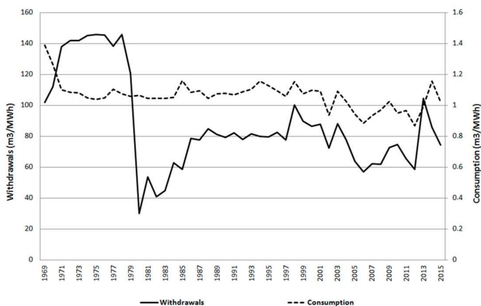
Figure 5. Evolution of technological water intensity in terms of water withdrawals (left axis) and water consumption (right axis) of thermal power stations in the Ebro River basin, 1969–2015. Note: The Escucha and Castelnou coal-fired power stations—using air-cooled condensers—are excluded. Source: own design (see ‘Data File S1’ in Supplementary Materials).
