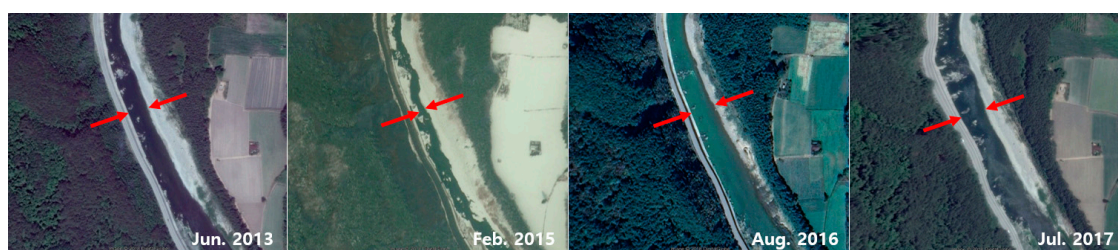
Figure 3. An example of a comparison of the top width of the main channel according to shooting time (from Google Earth Pro).
