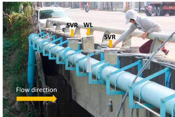
Figure 2. Photograph of the WL radar and two SVRs at Yenfong Bridge station.
