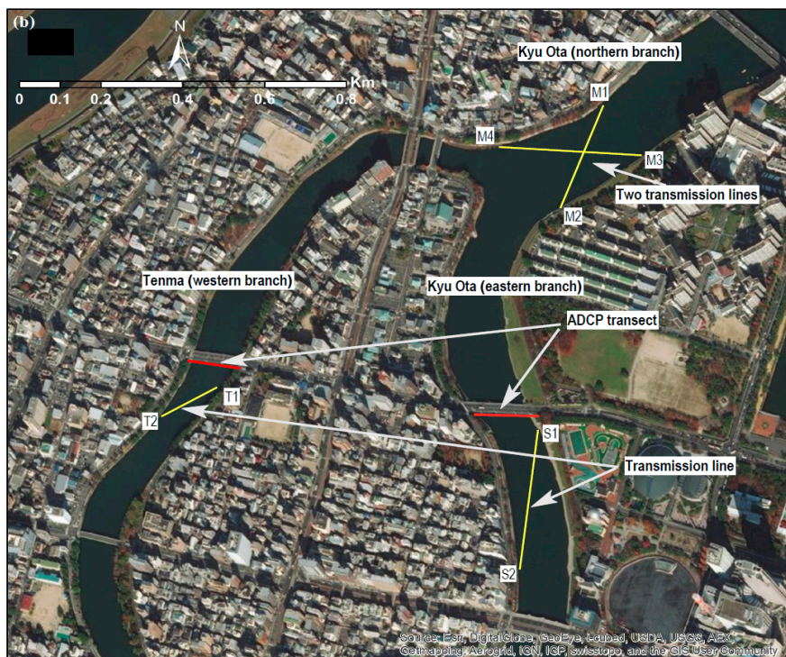
Figure 1. (a) Ota river channel network map. The black box denotes the study area. (b) Observation site and deployment of the fluvial acoustic tomography system (FATS) at the eastern, western, and northern branches. The yellow lines represent the transmission lines between the two transducers of FATS. S1–S2, T1–T2, and M1–M4 denote the locations of the transducers for FATS measurements. The red lines denote the acoustic Doppler current profiler (ADCP) transects for the comparison with FATS.
