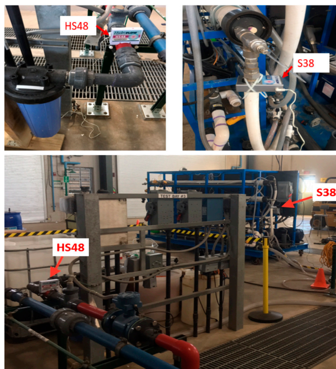
Figure 2. Installation points of the HydroFLOW devices. HS48 was installed in the metal pipeline before the cartridge filter. S38 was installed in the inlet of the RO vessel.
