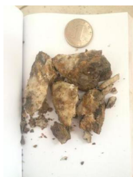
Figure 4. Sample of rock taken from the fractures in the tunnel. The soluble salt filling can be easily seen.
