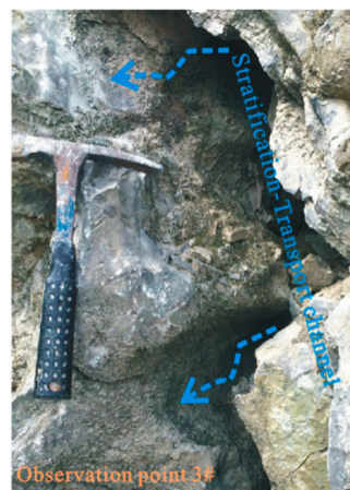
(d) Stratification strong dissolution to form a good water-guiding channel near Xiangshuidong.
