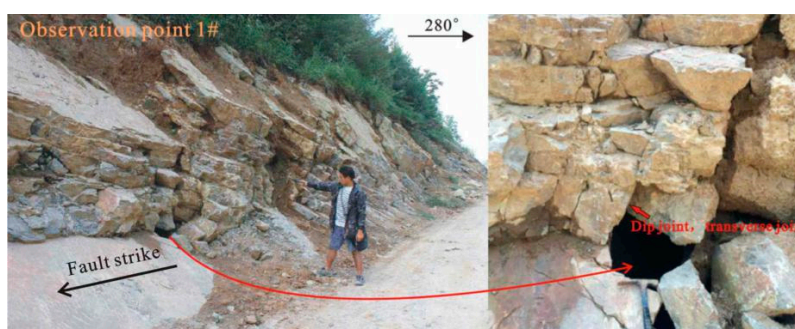
(a) The vertical hole group formed by the intersection of the Jialingjiang Formation and the vertical and horizontal joints was filled.
