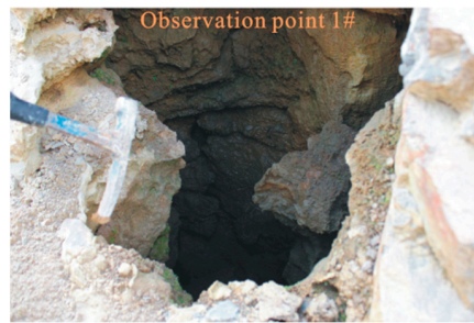
(b) Stress rotation: the original rock layer is subjected to tendency joints, cross-section cutting into blocks, and then dissolution into vertical holes.
