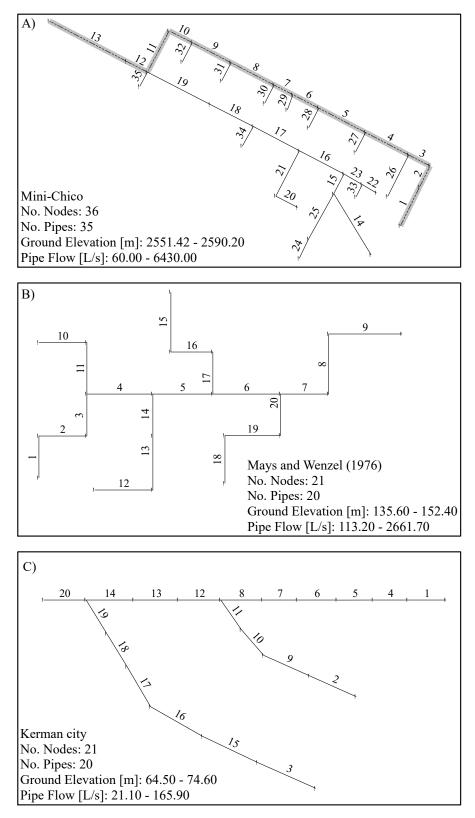
**Figure 1.** Sewer networks used for the analyses: (**A**) Mini-Chicó network; (**B**) Mays and Wenzel [13] network and (**C**) Kerman city network.
