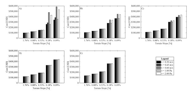
**Figure 3.** Network costs for the five wastewater proposed simulations: (**A**) Simulation 1 (Inflow per node 1 L/s), (**B**) Simulation 2 (Inflow per node 2 L/s), (**C**) Simulation 3 (Inflow per node 3 L/s), (**D**) Simulation 4 (Inflow per node 5 L/s), and (**E**) Simulation 5 (Inflow per node 10 L/s). Cost in (USD).
