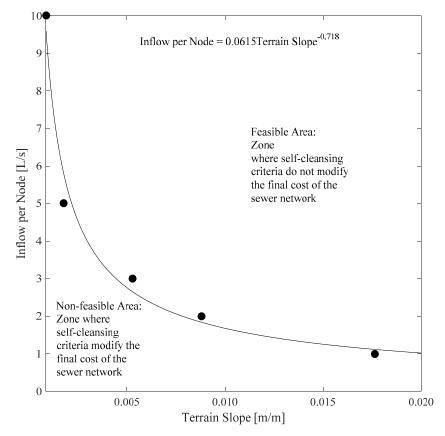
Figure 4. Self-cleansing limits in sewer systems.
