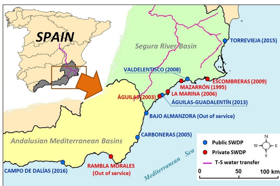
Figure 1. Location of seawater desalination plants (SWDPs) supplying water for agriculture in Southeastern Spain (SE Spain). State-owned SWDPs are shown in blue and private ones in red. Figures in brackets indicate the installation date and those that are currently out of service. The Tajo–Segura (T–S) water transfer system is also depicted in purple.
