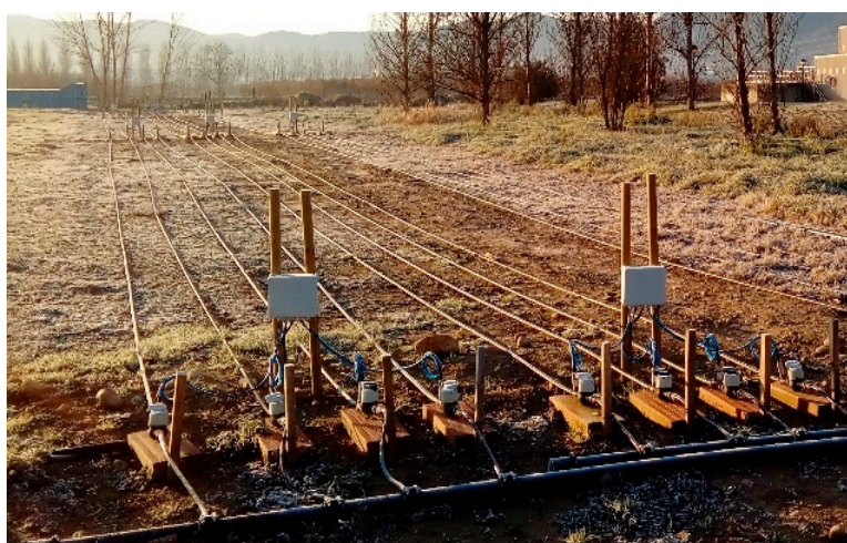
Figure 2. View of the pressure transducers and water meters of the irrigation subunits.
