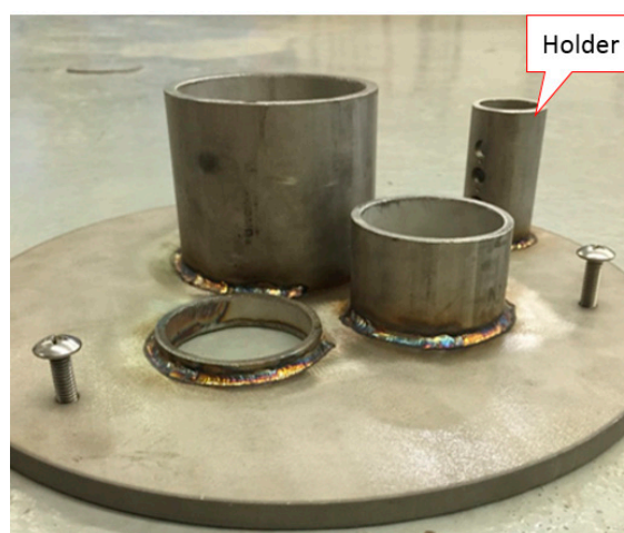
Figure 3. The orifice insert with three vertical pipes and one perforated pressure transducer holder.
