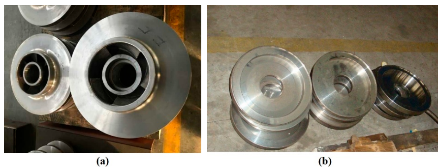
Figure 2. The main flow passage components including (a) the impeller and (b) the guide vane.
