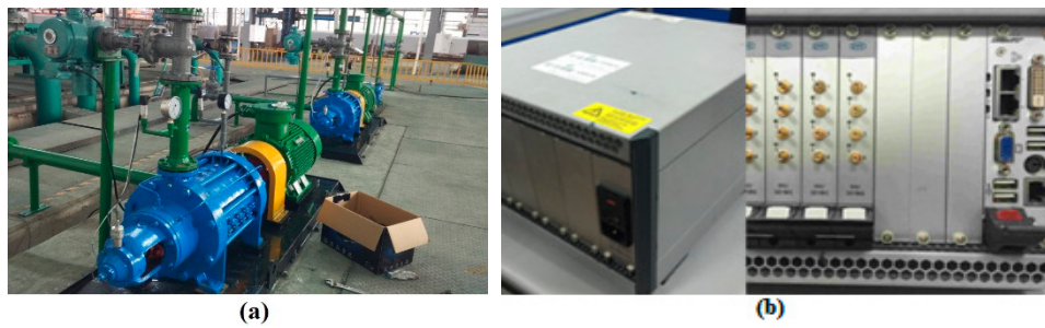
Figure 5. The test system including (a) the pump circulation system and (b) the INV3020C signal acquisition system.
