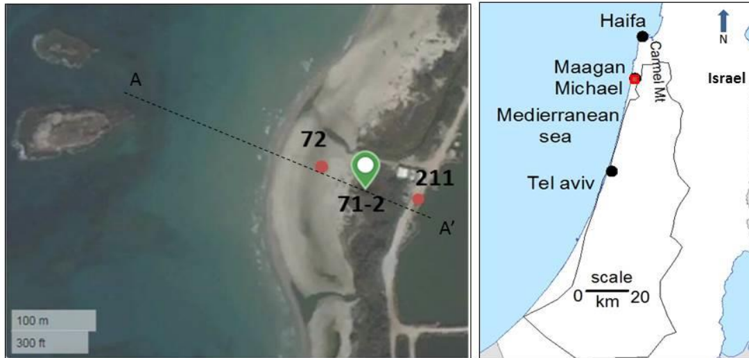
Figure 1. Location map site and a map of well location. Well 211 is a pumping well, while wells 72 and 71-2 are observation wells. The grey line on the right figure denotes the boundary of the basin of the Late Cretaceous Yarkon Taninim aquifer. Shown also is the location of geological cross section of Figure 2.
