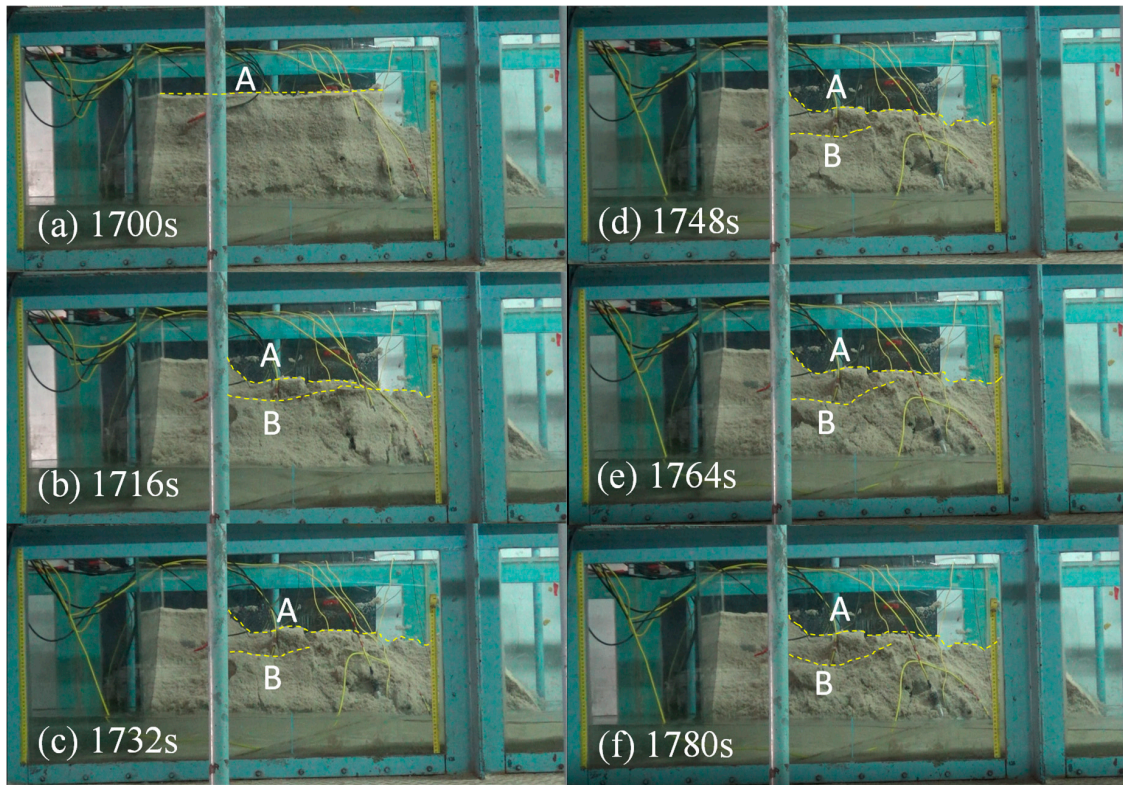
Figure 12. Before and after images of the successive slide (Event 3).
