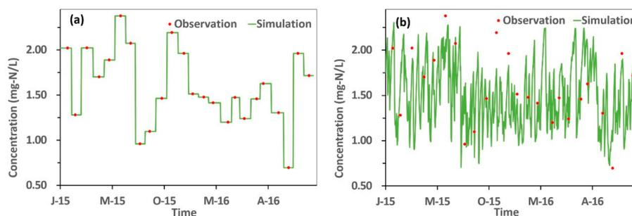
**Figure 2.** The model-fitted  $\text{NO}_3^-$  concentration of site no.1 for an unmeasured time sequence based on (a) a rectangular interpolation and (b) a simple linear regression model using functions in the loadflex package. The red points and green line stand for observations and concentration predictions, respectively.
