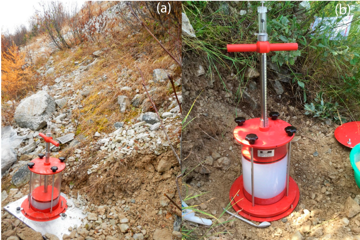
Figure S1. Balloon method device used in in situ soil unit weight measurements in gravelly soil at the scree slope. (a): densitometer testing in a steep section of the slope with support plate at the base (IGT design); (b): densitometer set up near IT4.
