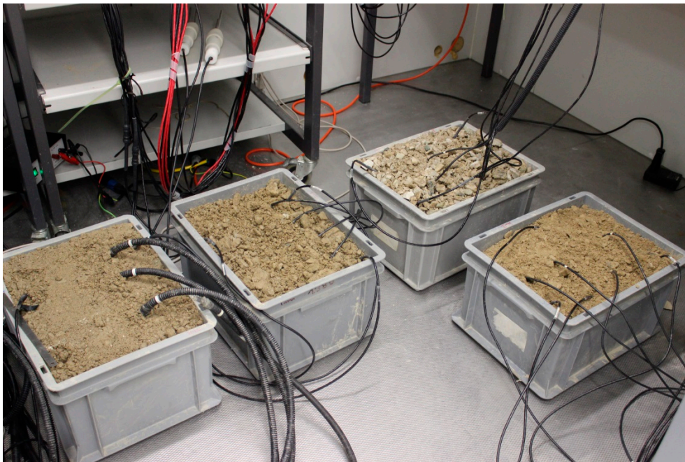
Figure S4. Soil in reconstituted samples for calibrating sensors from IT1-4.
