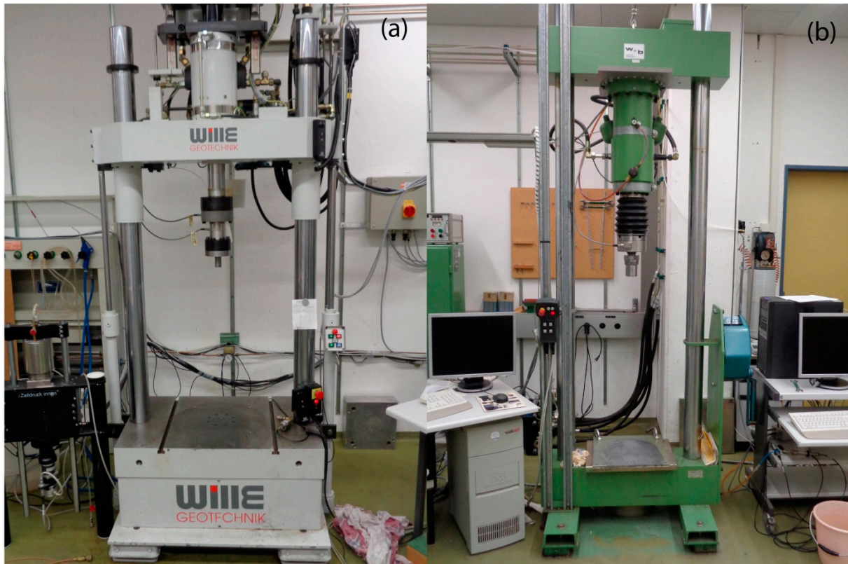
Figure S2. Triaxial testing apparatuses. (a): mid-scale; (b): large scale, (photograph: R. Grob, 2015).
