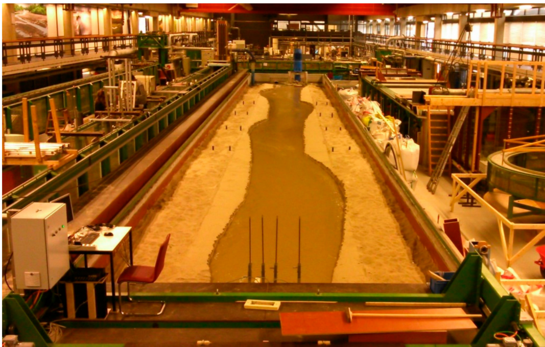
Figure 7. Alternate bars enhance opposite bank erosion (courtesy of Andrés Vargas-Luna).
