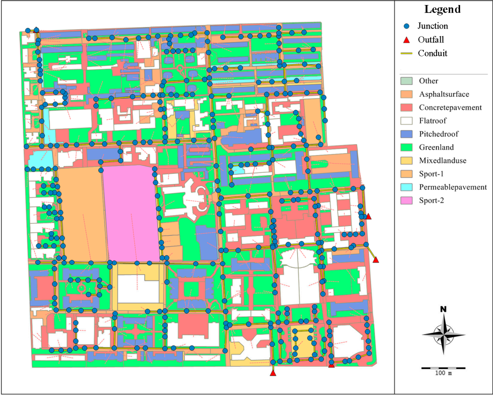
Figure S1 Network and areas covered by scenarios in the campus of Beijing Normal University
