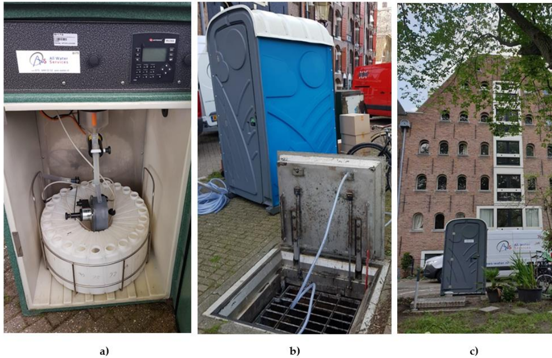
Figure S1. Photographs of wastewater sampling installation on Prinseneiland. From left to right, a) Automatic sampling cabinet with 24 sample bottles, b) Portable toilet that housed the sampling cabinet with sampling hose leading through the manhole cover to wet well below, c) View of sampling location once the installation of the sampler was completed.
