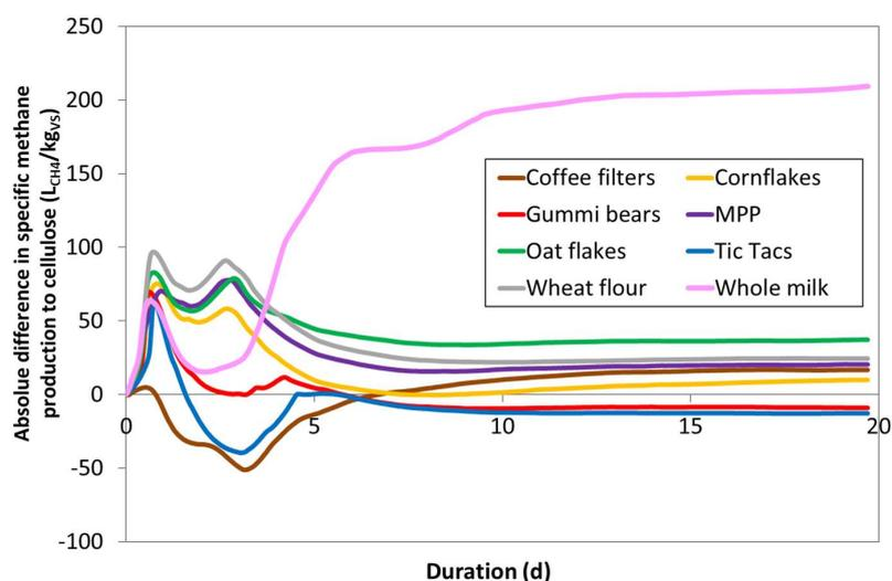
**Figure 3.** Absolute difference in the specific methane production relative to microcrystalline cellulose of the eight alternative positive control substrates tested.
