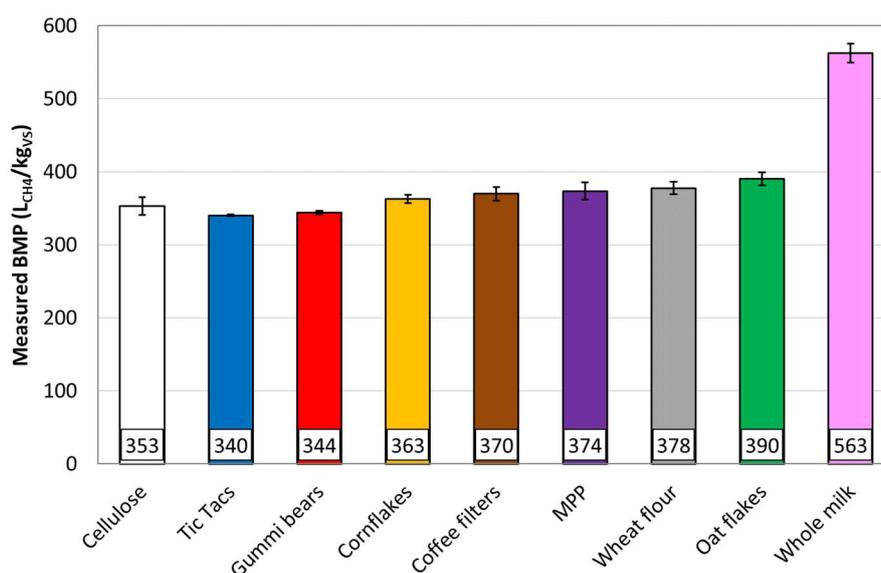
**Figure 5.** Measured BMP for microcrystalline cellulose and alternative positive control substrates. Error bars indicate standard deviation ( $n = 9$  for microcrystalline cellulose and  $n = 3$  for all other substrates). Values have been sorted in ascending order.
