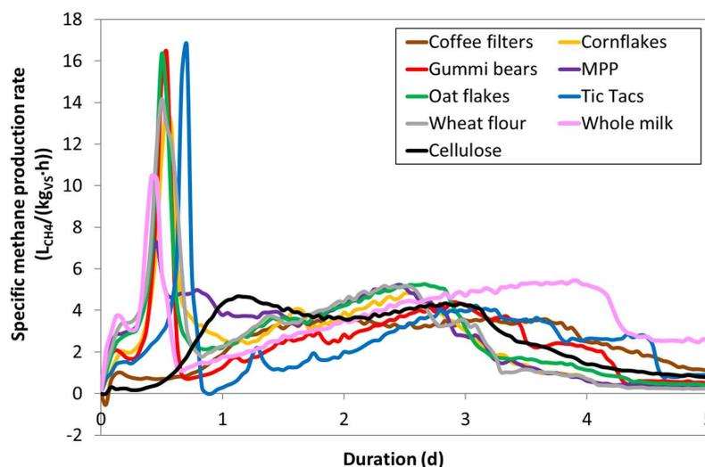
**Figure 2.** Average specific methane production rate of microcrystalline cellulose ( $n = 9$ ) and the eight alternative positive control substrates ( $n = 3$ ) tested in the first 5 days of incubation.
