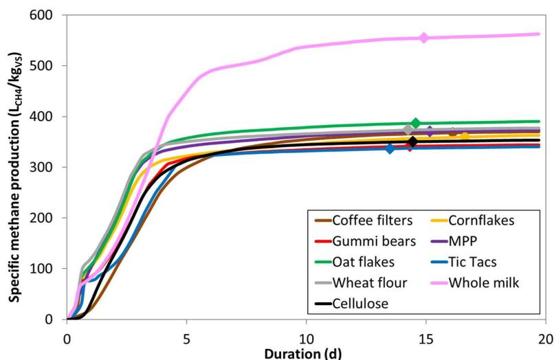
**Figure 1.** Average specific methane production of microcrystalline cellulose ( $n = 9$ ) and the eight alternative positive control substrates ( $n = 3$ ) tested. Diamonds indicate the time when the daily gas production was below 1% of cumulative production during three consecutive days.
