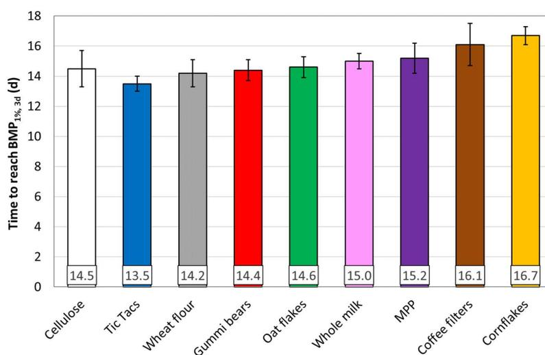
**Figure 4.** Time to reach the termination criterion  $BMP_{1\% \text{ net}, 3d}$  for microcrystalline cellulose and alternative positive control substrates. Error bars indicate standard deviation ( $n = 9$  for microcrystalline cellulose and  $n = 3$  for all other substrates). Values have been sorted in ascending order.
