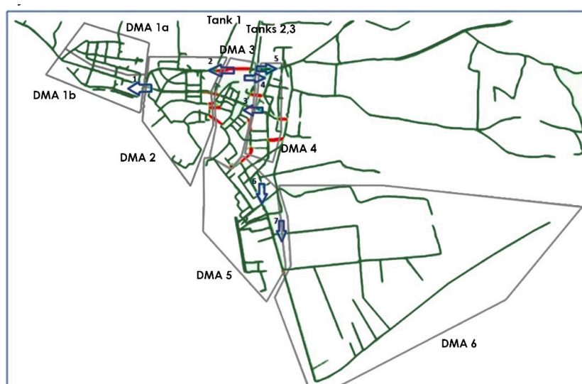
Figure 2. District Metered Areas (DMAs) formation based on the optimal pressure at the critical node of each DMA.
