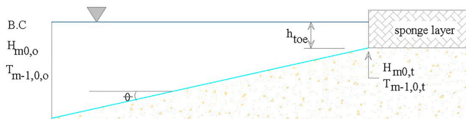
Figure 3. Wave parameters at toes in SWASH model for case studies.
