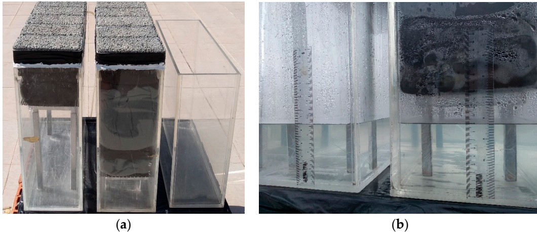
Figure 4. Model systems exposed to rain events. (a) Model systems and the control box; (b) Infiltrated rainwater measure.
