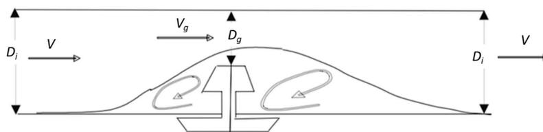
Figure 4. Parameters involved in calculating minor loss for online type emitters [7].
