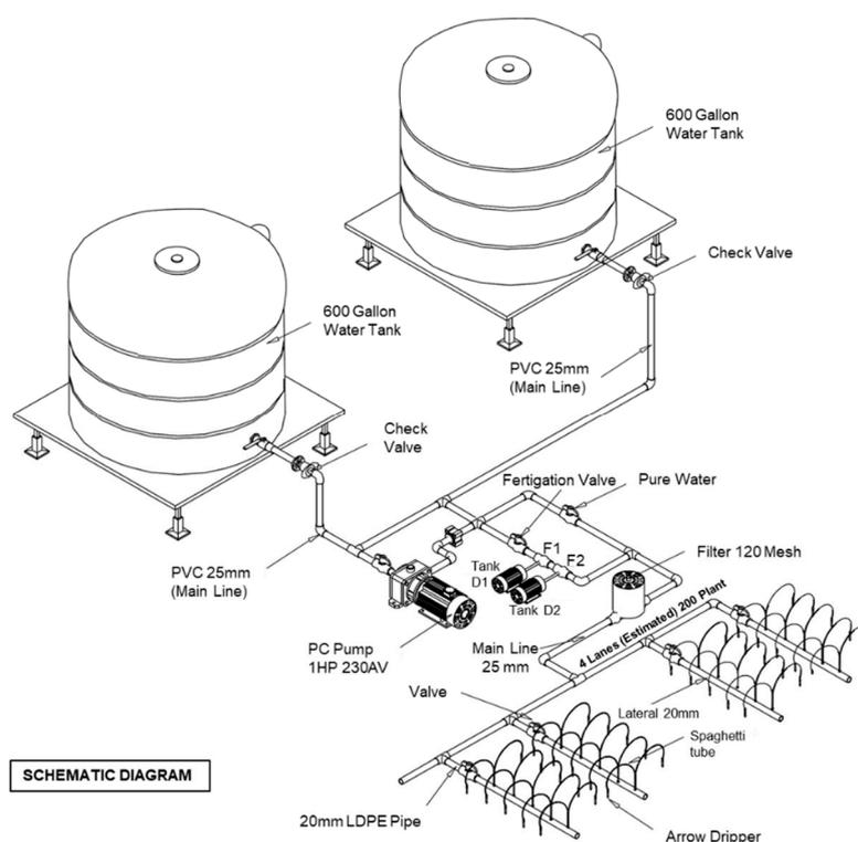
**Figure 2.** Overall drip irrigation system components.
