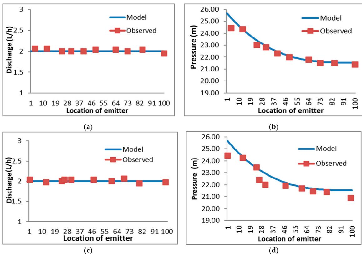
**Figure 5.** Comparison between measured and modelled discharges and pressures at emitters in lateral pipe 1 and lateral pipe 2. (a) Discharge at emitters on lateral pipe 1; (b) Pressure at emitters on lateral pipe 1; (c) Discharge at emitters on lateral pipe 2; (d) Pressure at emitters on lateral pipe 2.
