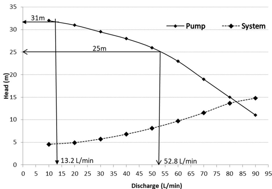
Figure 7. System curve and pump curve of the existing drip irrigation system.
