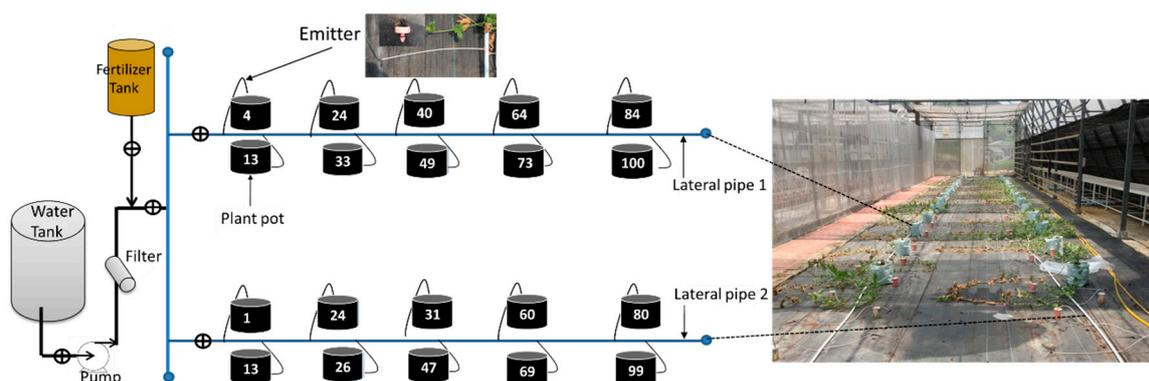
**Figure 3.** Emitter locations for the measurement of pressure and flow rate. The numbers in the planter pot indicate the plant pot numbers where the measurements were done. Photos in the diagram show the spaghetti emitter used in the existing system. Each lateral pipe has 100 emitters.
