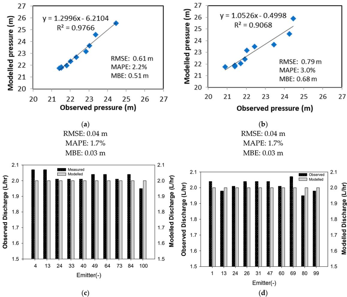
**Figure 6.** Modelled and observed pressure (upper) and discharge (lower) on lateral pipe 1 and lateral pipe 2. (a) Pressure on lateral pipe 1; (b) Pressure on lateral pipe 2; (c) Discharge on lateral pipe 1; (d) Discharge on lateral pipe 2.
