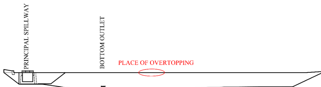
Figure 6. Longitudinal section of the Pocheň dam with an indicated place of overtopping.
