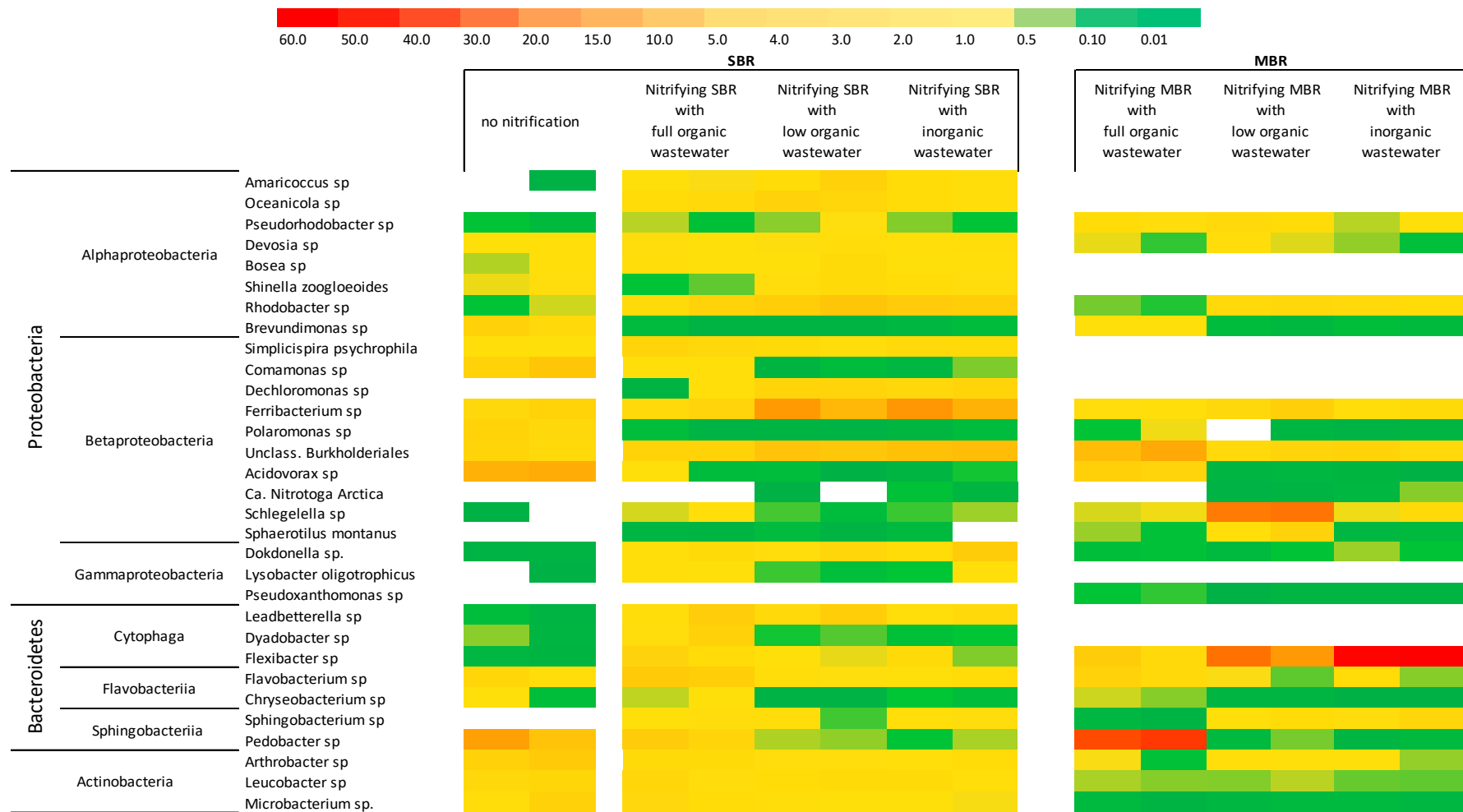
Figure 8. Dynamics of the most abundant bacterial genera in SBR and MBR pilot reactors before and after the change of carbon source in wastewater.
