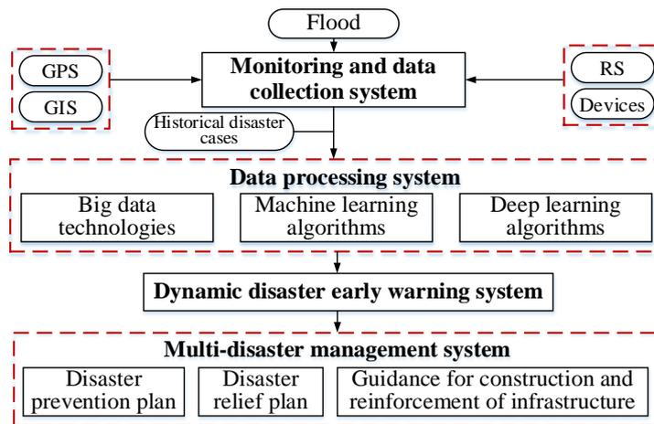
**Figure 9.** Multi disaster collaborative early warning system. GPS, global positioning system; GIS, geographical information system; RS, remote sensing.
