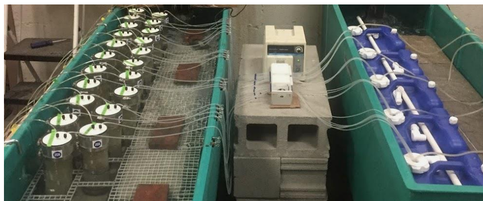
Figure S2. Flow-through sediment core incubation setup used in this study. Cores and source water were maintained at ambient lake temperature using controlled-temperature water bath tanks.
