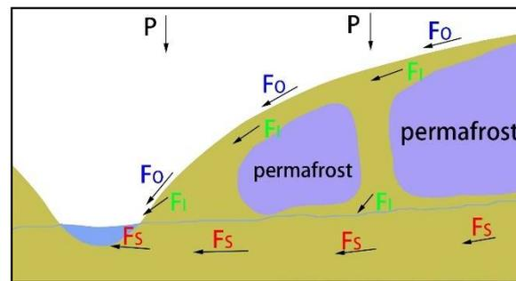
**Figure 2.** Schematic in-stream flow generation mechanisms in permafrost catchments (P: precipitation;  $F_0$ : overflow;  $F_1$ : interflow;  $F_s$ : saturated flow).
