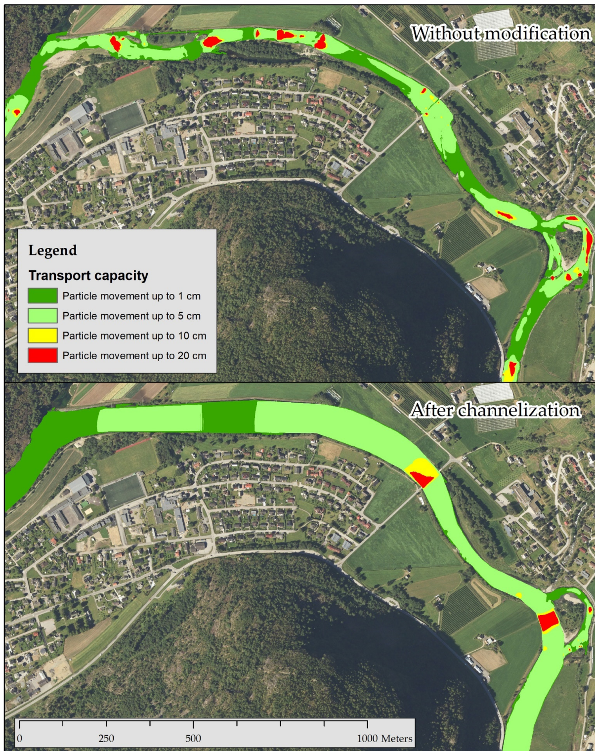
Figure 9. Map of particle movement according to shear stress with flow of 65 \text{ m}^3/\text{s} .
