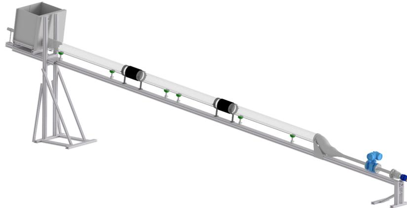
**Figure 2.** 3D CAD view of the reduced scale model (scale 1:20) used for the investigation of the air entrainment during the emptying of the forebay tank and the head race tunnel.
