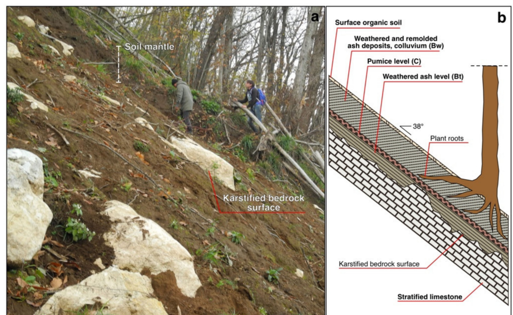
Figure 2. (a) Avalanche/erosion zone of the 21 December 2019 landslide and (b) schematic profile of a typical slope of the high-elevation zones of the Campania region (soil mantle thickness is exaggerated); modified from Reference [13].
