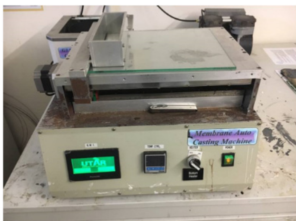
(a) Flat sheet membrane casting
