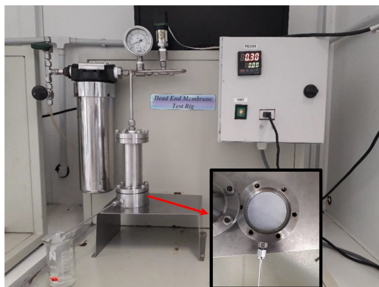
Figure 4. Dead-end test (pure water permeation set-up).
