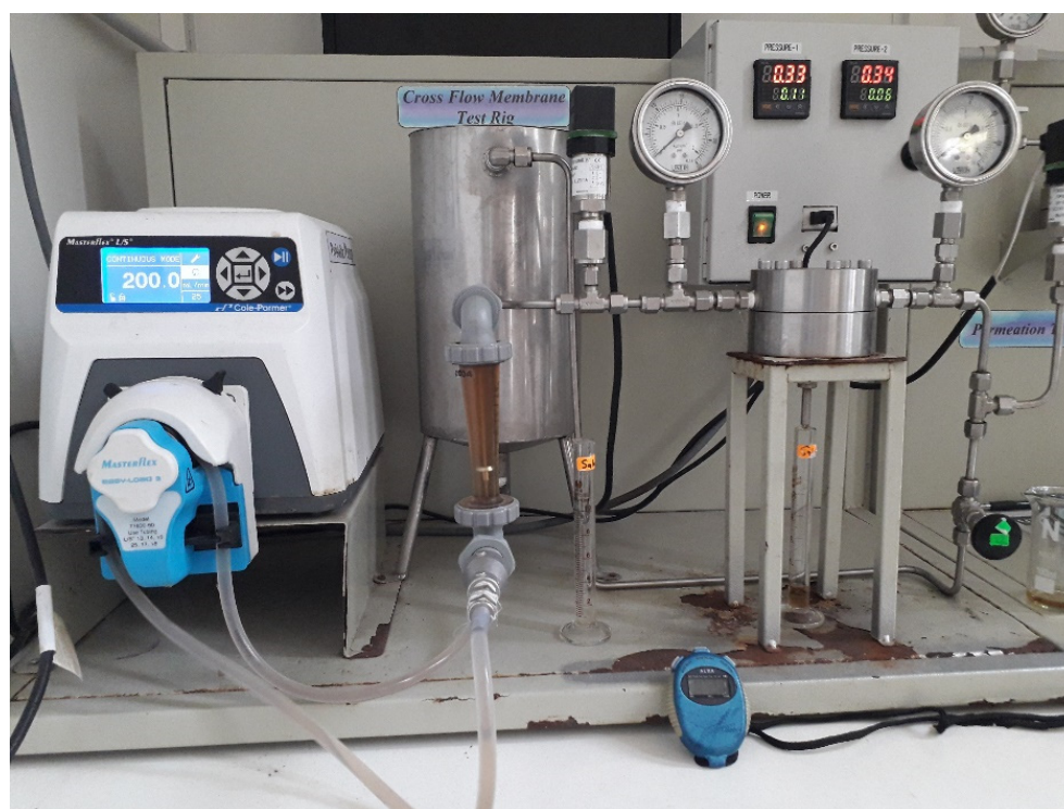
Figure 3. CFR test configuration (filtration treatment set).
