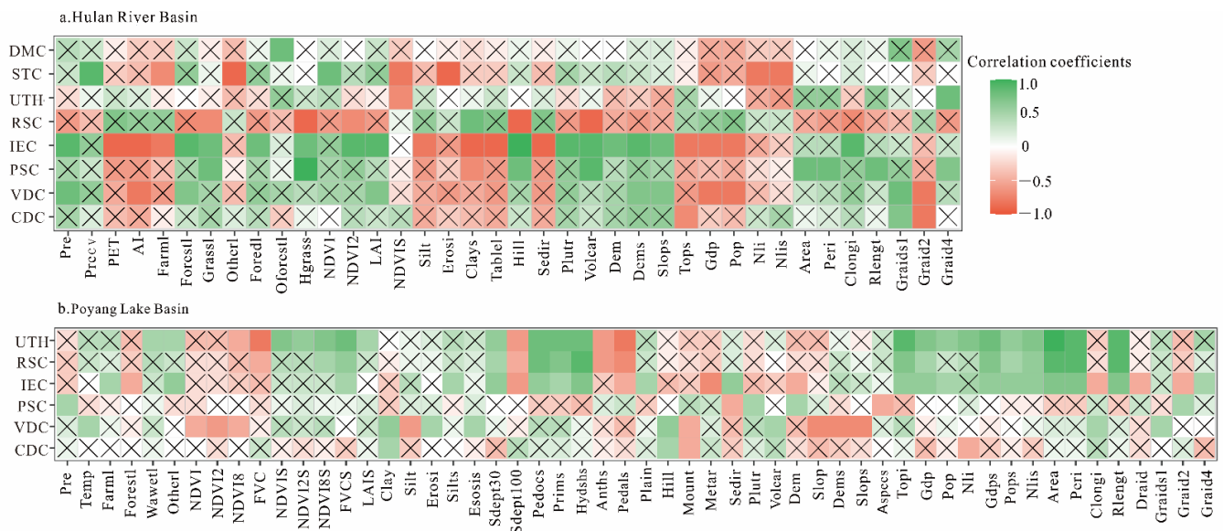
Figure 7. Correlation coefficients of model simulation efficiency (CDC for calibration period, VDC for validation period), hydrological model parameters, and indices of climate and underlying surface for the Hulan River Basin (a) and Poyang Lake Basin (b).
