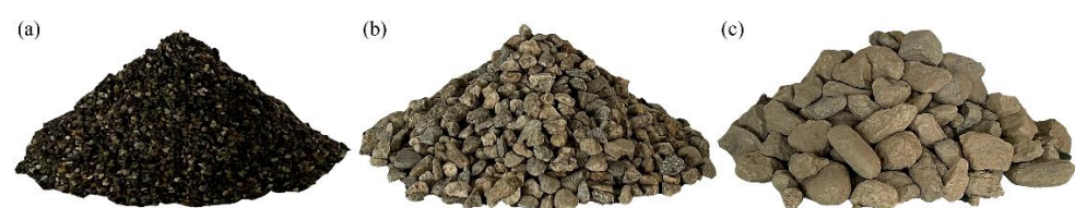
Figure 3. Sediments used in the experimental runs: (a) d_{50} = 1.53 \text{ mm} ; (b) d_{50} = 6.49 \text{ mm} ; (c) d_{50} = 17.98 \text{ mm} .
