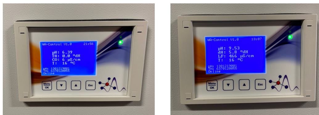
Figure 3. Measurement values of the WA-control. (Left): Reading values of the initial water (starting point for the production of the base model water) taken some minutes after filling the empty storage tank from the RISE in-house purified water supply; (Right): Typical reading values during the accelerated wear tests (values taken on 24 August 2020).
