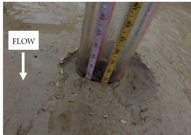
Figure 5. Scour hole development and the soil removal erosion pattern at the wake zone of the pier: run 14, V = 80.10 cm/s, WC = 38.12\% .
