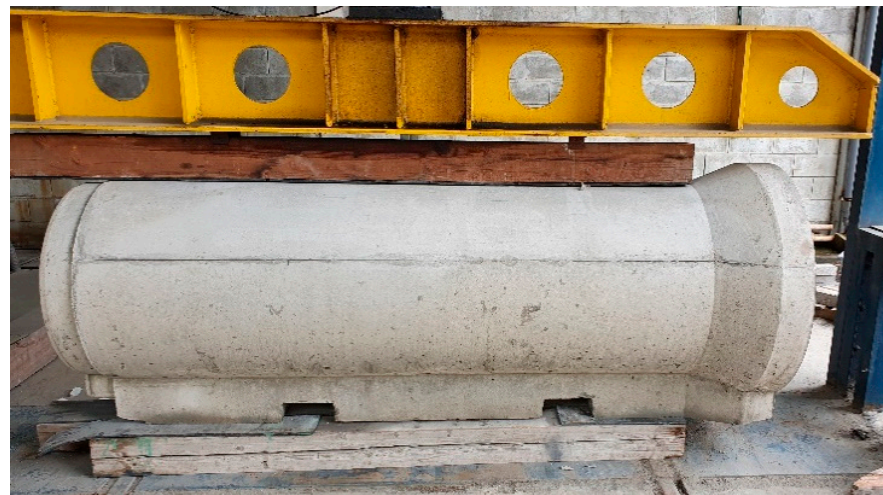
Figure 12. Three edge bearing test for complex cross-section reinforced concrete pipe.
