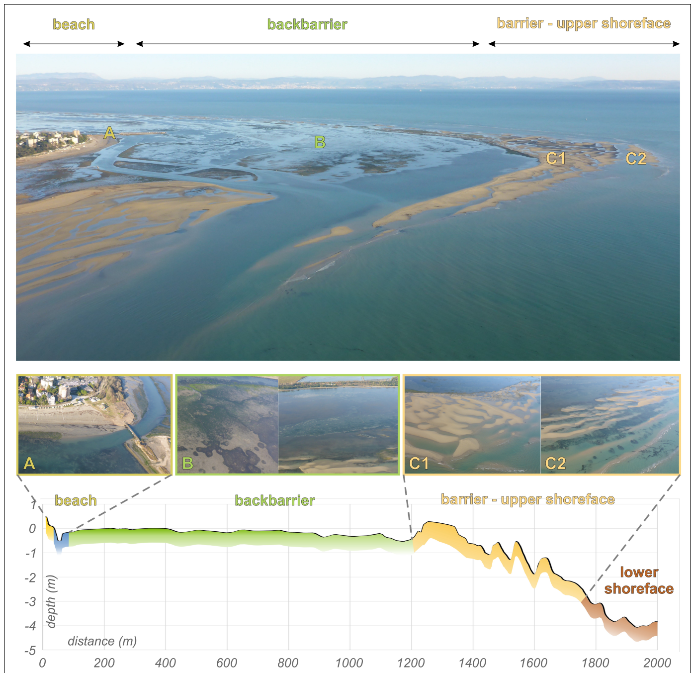
Figure 3. Morpho-bathymetric structure of the Mula di Muggia Bank. The barrier (C1) and the longshore bars (C2) migrate westward (from the top to the bottom of the upper image), thus obstructing the canal that crosses the backbarrier (B). The canal is the sole route for small boats to traverse the shallow silty zone toward the coastline (A) and the Grado Pineta marina.
