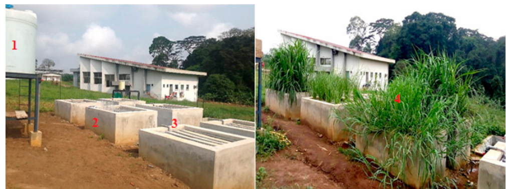
Figure 1. The experimental setup of the study; (1) feeding tank, (2) pilot VFCW beds, (3) inlet feeding pipes, (4) plant growth in the pilot beds two months after planting.
