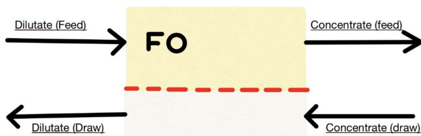
Figure 6. Forward osmosis process principle.
