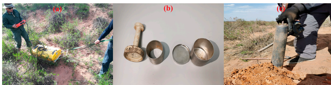
Figure 3. Real shots of the sampling tools and sampling process. (a) The staff are conducting radar detection. (b) The cutting ring and aluminum box used for sampling. (c) Luoyang shovel.
