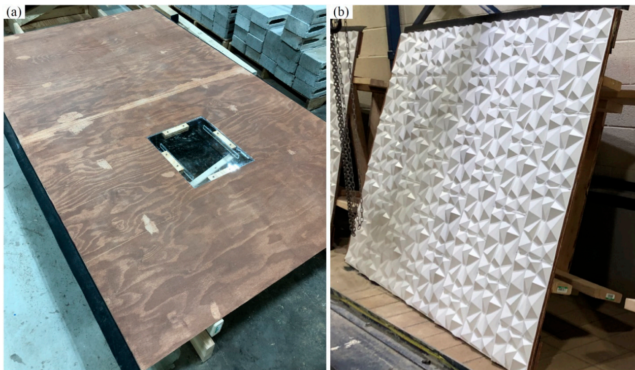
Figure 3. Bottom surface of the ice cover: (a) smooth condition, and (b) rough condition.
