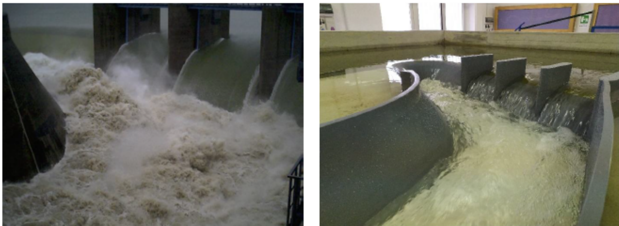
Figure 9. Comparison between the 2003 flow event (on the left) and the model scale reproduction (on the right).
