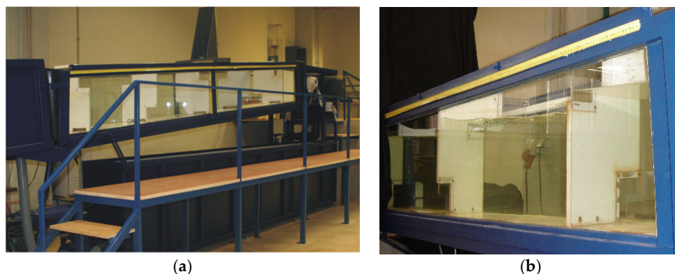
Figure 1. Experimental flume used (a) Side view of the flume; (b) Pool detail.
