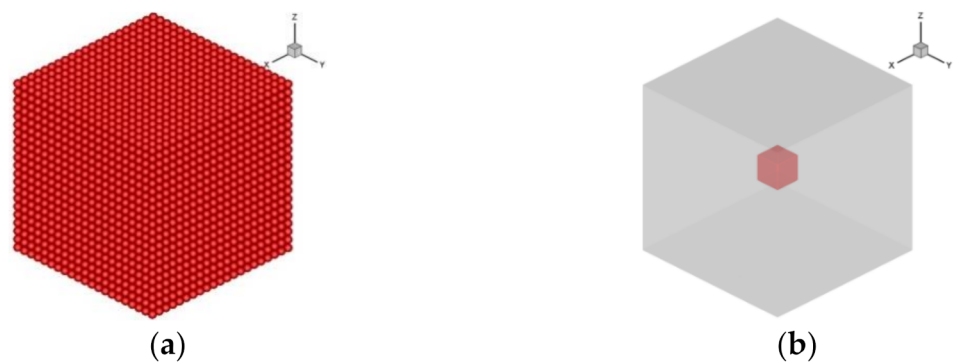
Figure 7. The computational model: (a) 1 m cubic fluid patch of MPS; (b) 7 m cubic air/1 m cubic water zone of VOF.
